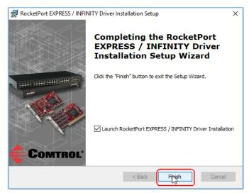
If you do not check this box, you can use the shortcut under the **Start** button at the location for your adapter type to start the driver installation: **Comtrol> RP EXPRESS INFINITY Driver Installation Wizard**
