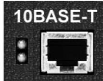
**Note:** Check the link polarity at the hub to make sure that there is Ethernet polarity at both ends of the Ethernet cable.
