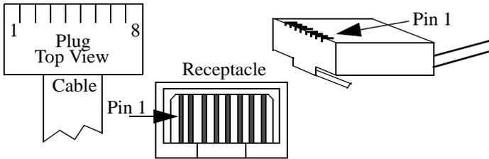
**Table 9. ISDN Port RJ45 Connector Pinouts**
