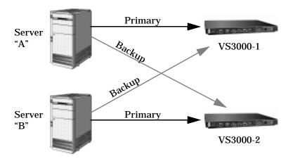
**Note:** VS-Link for Novell can support four VS3000 units (either primary, backup, or mixed) per Novell server. VS-Link for Windows NT can support thirty-two VS3000 units per NT server.
