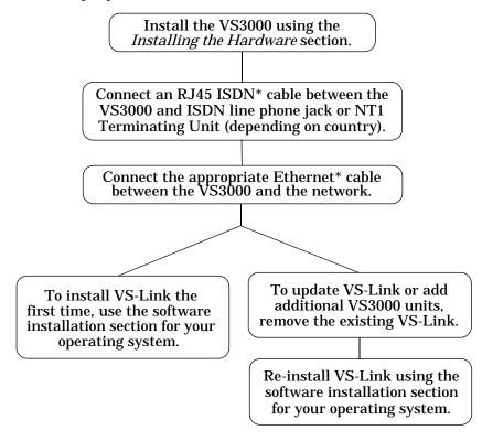
\* While ISDN and Ethernet cables may appear to be identical, they are not interchangeable. Make sure you are using the correct cable(s) in the correct locations.
