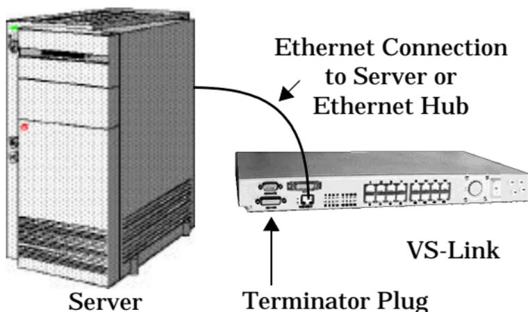
**Note:** Do not connect two VS1000 base units together. If connecting the VS1000 directly to the server, an **Ethernet crossover** cable is required. See the Installation and Configuration Guide for details.
