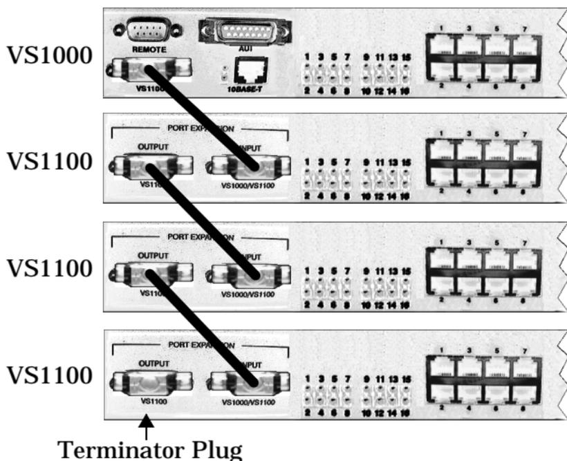
**Note:** *The VS1100 cannot be connected directly to the LAN. Remember, Ports 1 through 16 are RS-232 ports.*
