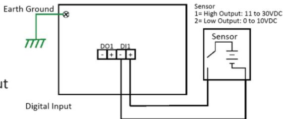
The DI supports isolated input circuit with digital high level input of 11VDC to 30VDC and digital low level input 0VDC to 10VDC. Do not apply a higher voltage than the specification; it may cause internal circuit damage or cause an incorrect DI action.
