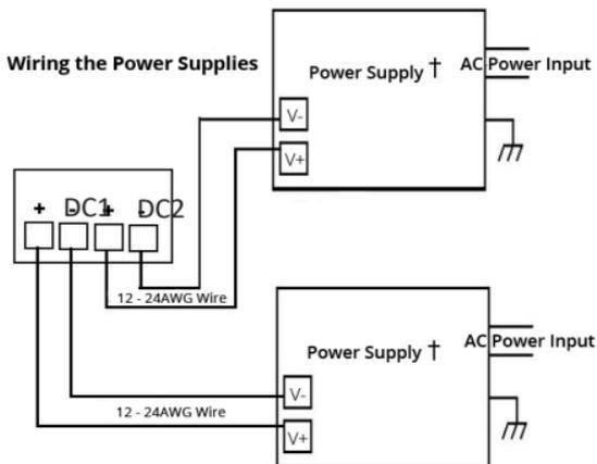
3. Insert the positive and negative wires (12 to 22 AWG) into the V+ and V- contacts.
