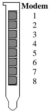
A four-modem version of the RocketModem card is also available. The four-modem version uses the same mounting bracket and connector block as the eight-modem version, but Jacks 5 through 8 are blocked with blank plugs.
