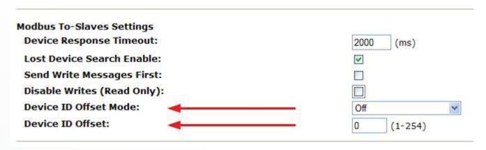
Device ID Offset Mode options include: Off, Add-To-Msg-ID, Subtract-From-Msg-ID.
