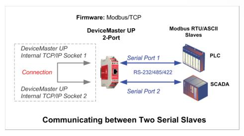
Note: Serial connections could be made with a 4-Port DeviceMaster UP.
