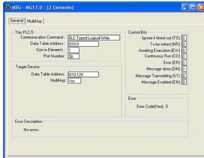
**6.6.10.7. SLC Typed Write - Set Transmit Produced Sequence Number Message**
