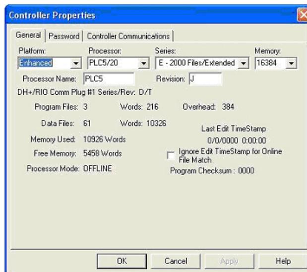
3. Select the **Controller Communications** tab and select the proper driver for RSLogix 5.
