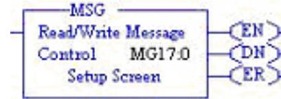
2. In the ladder logic, double-click the **Setup Screen** in the MSG instruction.
