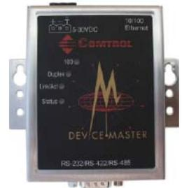
4. Verify that the **Status LED** has completed the boot cycle and network connection for the DeviceMaster is functioning properly using the table below.
