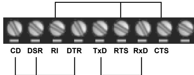
Wire the terminals together to create a loopback.
