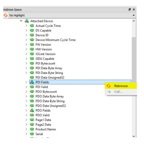
If you have the IODD loaded on your sensor(s), you'll be able to have more detailed information depending on your vendor. For example, under PDI Field, and Measured Value tag, you can view specific values regarding your device. You can also start using Byte Array, Byte String, etc to view your data.
