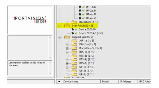
2. The IO-Link Master will appear on the bottom right of PortVision DX. Navigate to Software version and confirm its EIP / PNIO v1.5.0.1 or higher. Keep note of the IP Address – this'll be used in the next step.
