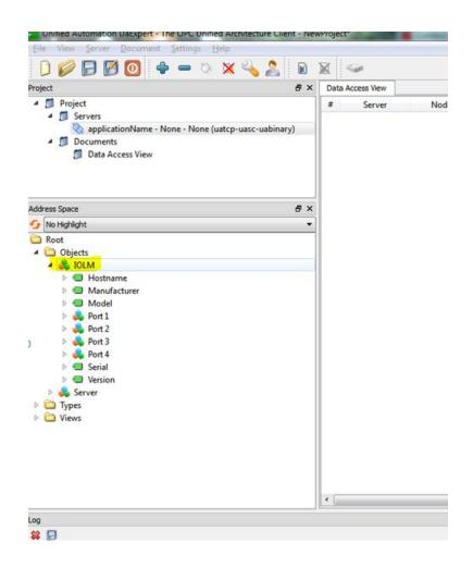
2. Expand one of your **Ports** that a sensor is attached to. In this example, a Leuze sensor (distance-measuring sensor) is attached to the port 2.
