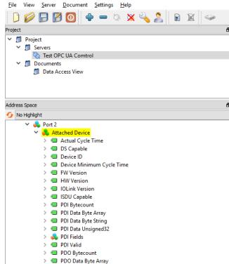
4. Now, you can explore the different tags and view whichever data you want. To test if the IO-Link Master is properly working with its respected sensor(s), click on Vendor Name tag (left side), then look over on the Attributes (right side). Under Value, the Vendor Name of our device (Leuze Electronic) for the port confirms that the Client, Server, and Port are all communicating – you can now freely view the data for whichever tag.
