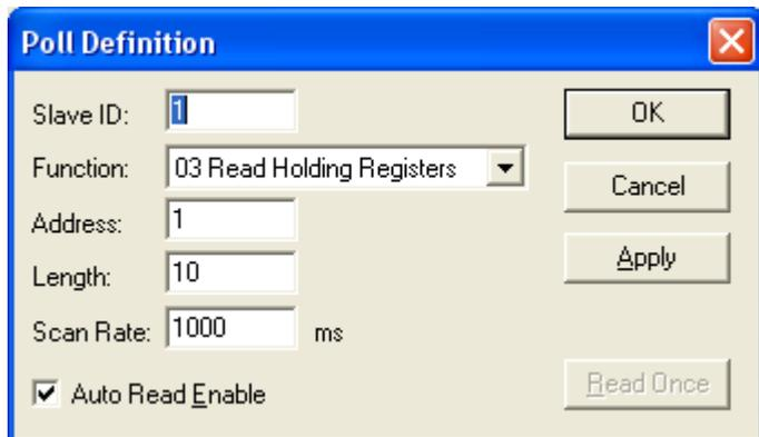
Change the default length of 10 to 40 to match the length field in the Modbus Slave application.
