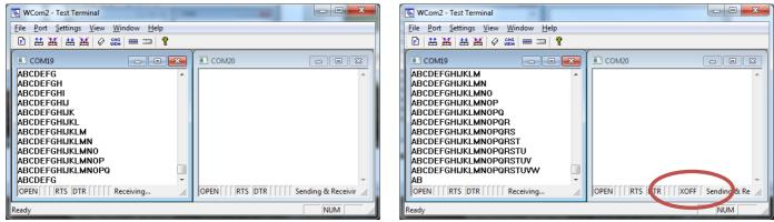
At this point the COM19 port should have the alphabet scrolling past in a 'sawtooth' type pattern.
