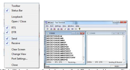
In COM20 Right Click and remove the checkmark on Send. The data should stop scrolling in COM19
