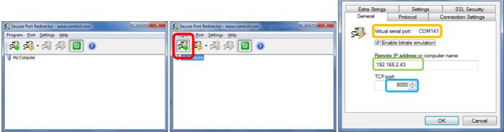
Launch SPR (Secure Port Redirector) and click the highlighted icon to add a new com port. Select a com port number (we will use 141 through 144) using the drop down arrow.
