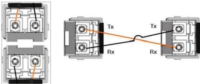
**Note: This is a Class 1 Laser/LED product. Do not stare at the Laser/LED beam. The SFP port does not function until the fiber cable is linked to another active device. The SFP and corresponding RJ45 ports work in an exclusive mode. Traffic sent or received through the SFP module will have priority, thus no traffic will be sent or received over the corresponding RJ45 connection. To use the RJ45 connection, remove the corresponding SFP.**
