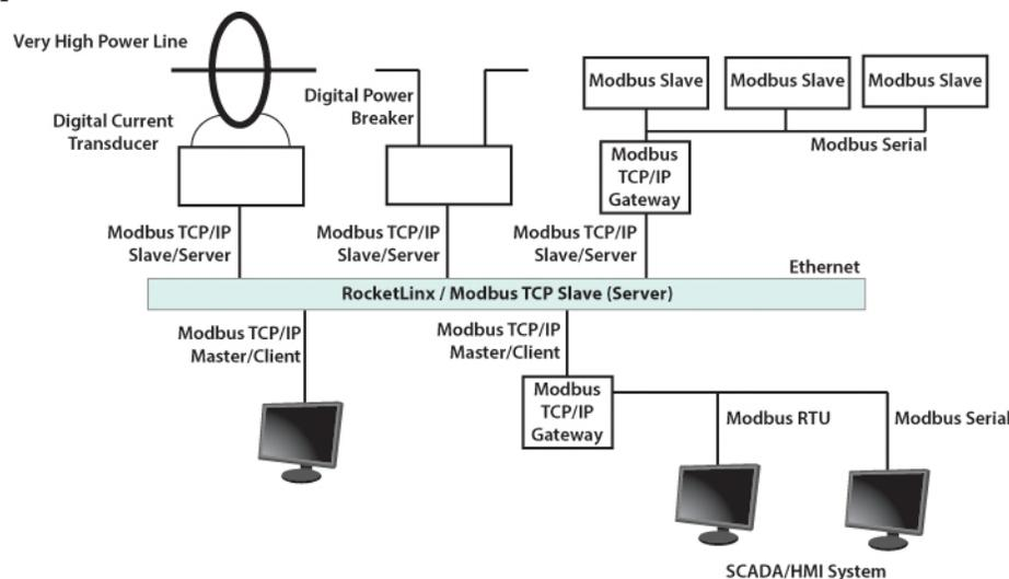
The ES8509-XT operates as slave/server device, while a typical master/client device is a host computer running appropriate application software, for example, a SCADA / HMI system. The ES8509-XT can be polled through Ethernet, thus the Modbus TCP/IP master can read or write to the Modbus registers provided by the Modbus TCP/IP.
