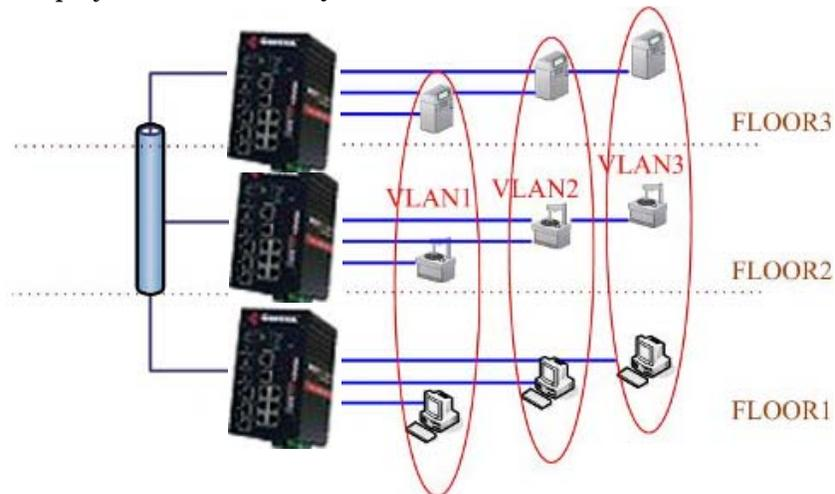
The ES8509-XT supports VLAN tunneling (QinQ), which expands the number of VLANs by adding a tag to the 802.1Q packets. The original VLAN is usually identified as Customer VLAN (C-VLAN) and the new VLAN is Service VLAN(S-VLAN). By adding the additional tag, QinQ increases the possible number of VLANs. After QinQ is enabled, the ES8509-XT can reach up to 256x256 VLANs. With different standard tags, it also improves network security.
