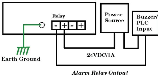
The failure events are selectable and enabled using the DIP switch on the ES8105. The relay contacts are rated for a maximum of 1A at 24VDC.
