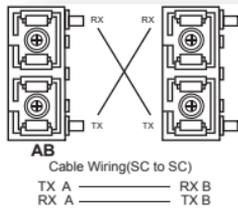
A wrong connection will cause the fiber port not to work properly.
