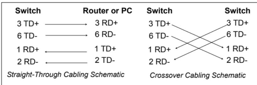
The LINK/ACT LED is lit when the cable is correctly connected. The LINK/ACT LED is lit yellow for a 10BASE-TX Ethernet connection or green for a 100BASE-TX Ethernet connection. Always make sure that the cables between the switches and attached devices (for example, switch, hub, or workstation) are less than 100 meters (328 feet).
