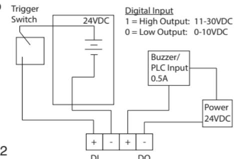
external DC type signal input and can be configured to send alert message through Ethernet when the signal is changed.
