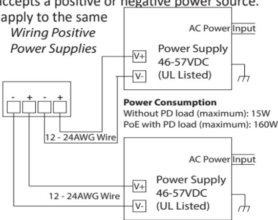
Positive and negative power system inputs are both accepted, but PWR1 and PWR2 must be in the same mode.
