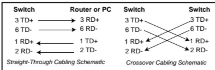
The Ethernet cables use Pins 1, 2, 3, and 6 of an 8-pin RJ45 connector. The signals of these pins are converted by the automatic MDIX function, as shown in the following table.
