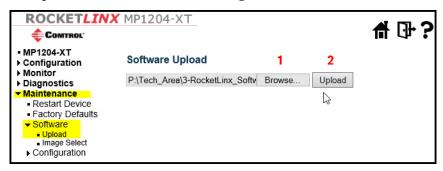
Note: While the firmware is being updated, Web access appears to not be functioning. The front LED flashes Green / Off with a frequency of 10 Hz while the firmware update is in progress. Do not restart or power off the device at this time or the switch may fail to function afterwards.
