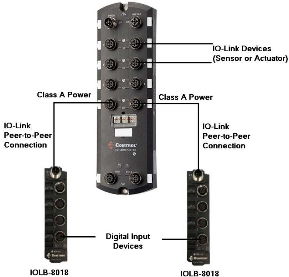
The connected IO-Link devices have individual parameter information detected during automatic scanning with the Comtrol IO-Link Master. Refer to [Configuring the IOLB-8018](#) on Page 15 for more information.
