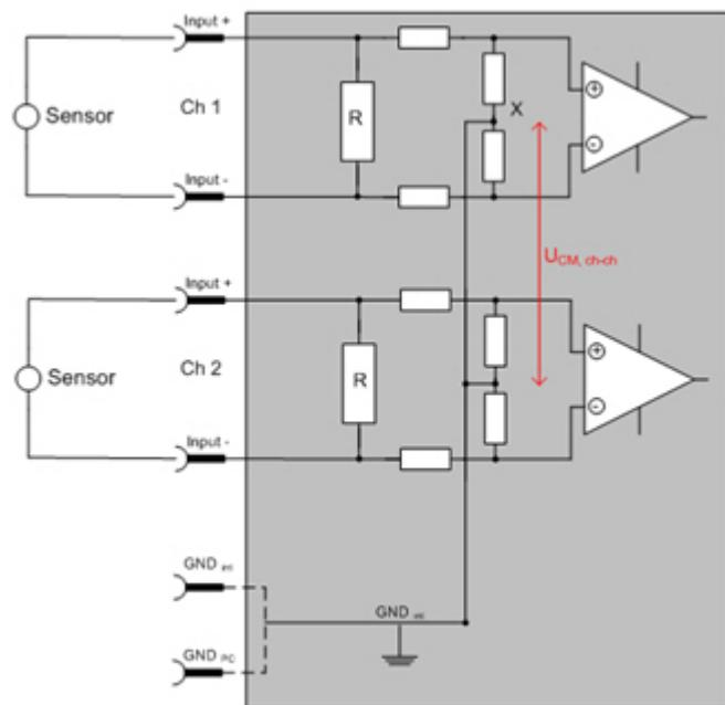
**Note:** Dashed lines indicate that the respective connection may not necessarily be present in each DIFF module.
