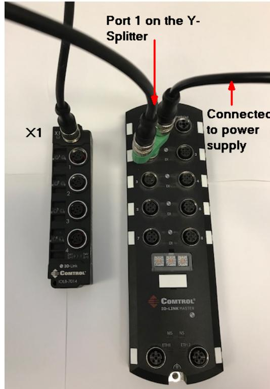
5. Apply power to the 24V power supply connected to the IOLB-7014.
