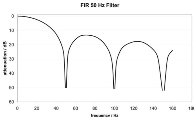
**Note:** Typical attenuation curve of notch filter at 50 Hz
