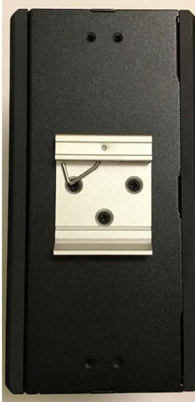
2. Hook the unit onto the DIN rail.
