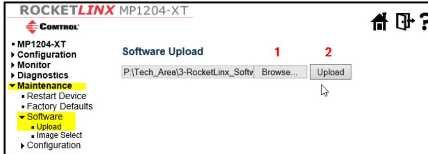
**Note:** While the firmware is being updated, Web access appears to not be functioning. The front LED flashes Green / Off with a frequency of 10 Hz while the firmware update is in progress. **Do not restart or power off the device at this time or the switch may fail to function afterwards.**
