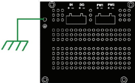
On the bottom side of the ES8509-XT, there is one earth ground screw. Loosen the earth ground screw with a screw driver, then tighten the screw after the earth ground wire is connected.
