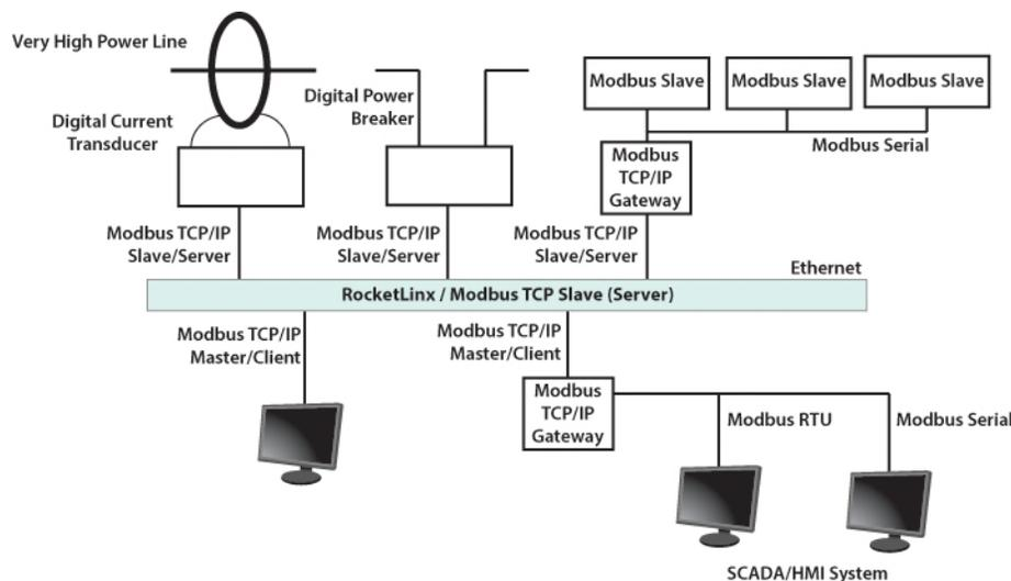
The ES7510-XT operates as slave/server device, while a typical master/client device is a host computer running appropriate application software, for example, a SCADA / HMI system. The ES7510-XT can be polled through Ethernet, thus the Modbus TCP master can read or write to the Modbus registers provided by the Modbus TCP.
