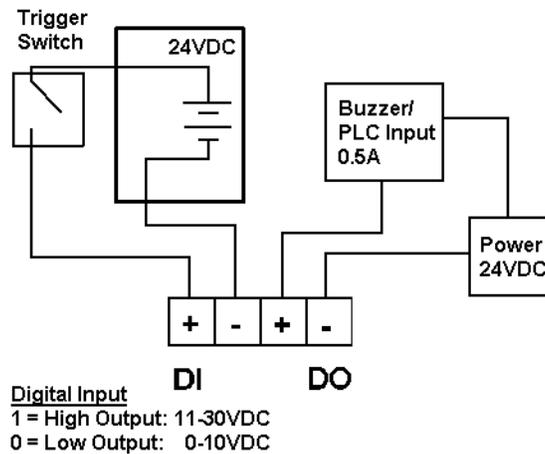
Digital output relay contacts are energized (open) for normal operation and close for fault conditions. The digital output relay contacts support up to 0.5A at 24VDC. Do not apply voltage and current higher than the specifications.
