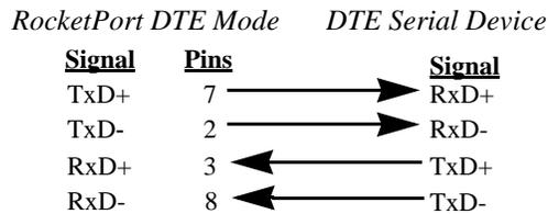
**Note:** RS-422 signals are not standardized and each serial manufacturer uses different pinouts. Refer to the serial device documentation to determine the pinouts for the signals above.
