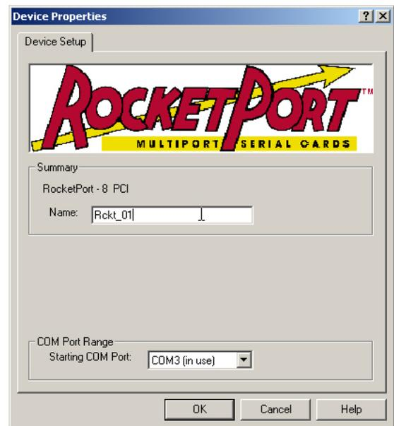
In addition, you can use **Starting COM Port** to set nonsequential starting COM port numbers for each adapter, thus leaving gaps in the COM port numbering sequence.
