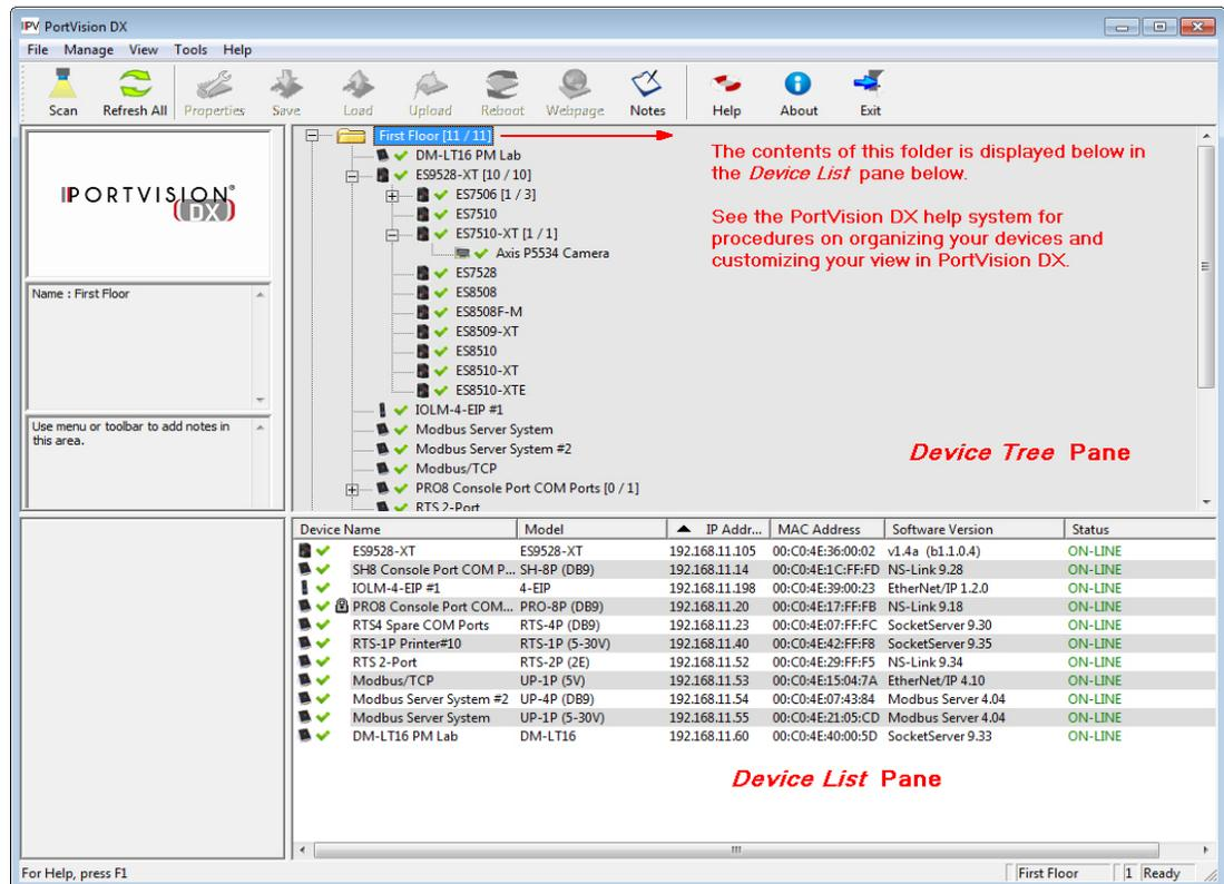
See the PortVision DX Help system for detailed information about modifying the view. For example, the above screen shot illustrates devices layered in folders.
