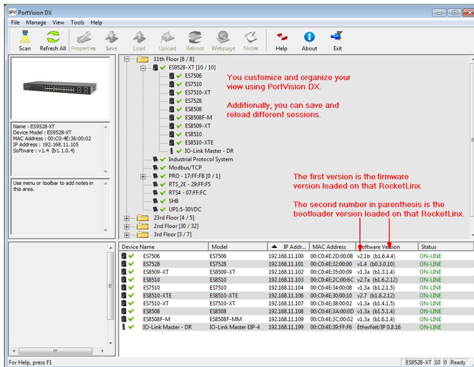
4. Check the [Control download](#) site for the latest firmware and bootloader. Simply, click your product type and click the **Software** link and check the latest version against the version on the ES8508. Use the next subsection for procedures to upload the firmware (web interface) and bootloader.
