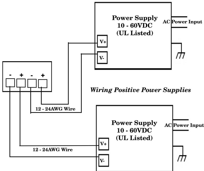
**Note:** Power should be disconnected from the power supply before connecting it to the switch.
