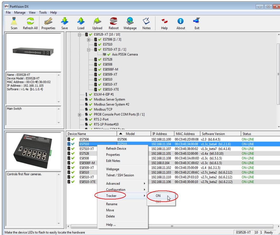
2. If necessary, you may need to click **Tracker** and **ON** several times to catch the flashing **SYS LED**.
