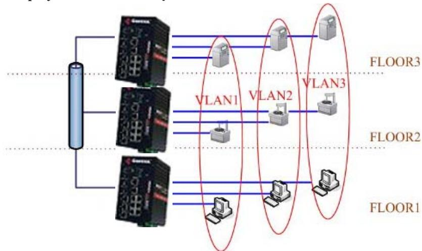
The ES8508 supports VLAN tunneling (QinQ), which expands the number of VLANs by adding a tag to the 802.1Q packets. The original VLAN is usually identified as Customer VLAN (C-VLAN) and the new VLAN is Service VLAN (S-VLAN). By adding the additional tag, QinQ increases the possible number of VLANs. After QinQ is enabled, the ES8508 can reach up to 256x256 VLANs. With different standard tags, it also improves network security.
