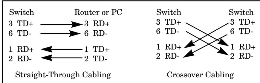
Connect one side of an Ethernet cable into any switch port and connect the other side to your attached device. The **LNK/ACT** LED is lit when the cable is correctly connected. Always make sure that the cables between the switches and attached devices (for example, switch, hub, or workstation) are less than 100 meters (328 feet) and meet these requirements.
