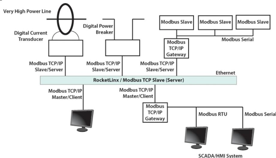
The ES8508 operates as slave/server device, while a typical master/client device is a host computer running appropriate application software, for example, a SCADA / HMI system. The ES8508 can be polled through Ethernet, thus the Modbus TCP/IP master can read or write to the Modbus registers provided by the Modbus TCP/IP.
