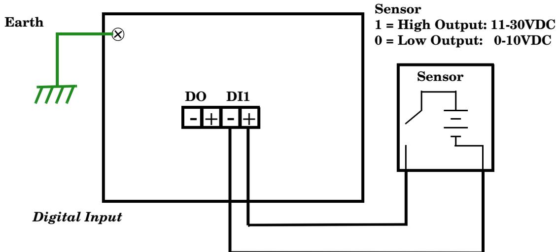
Digital output relay contacts are energized (open) for normal operation and close for fault conditions. The digital output relay contacts support up to 1A at VDC. Do not apply voltage and current higher than the specifications.
