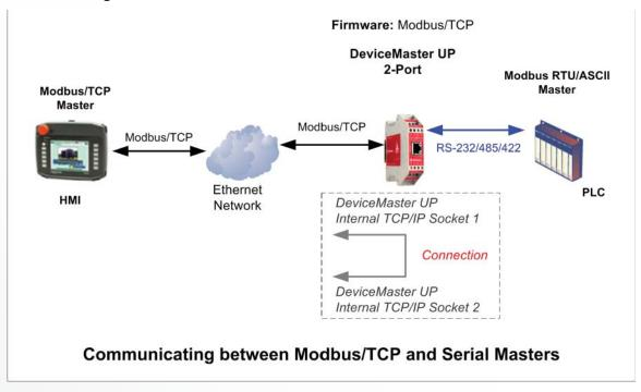
Note: Serial connections could be made with a 4-Port DeviceMaster UP.
