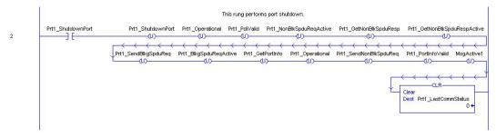
This rung clears all flags necessary to cleanly shut down a port.
