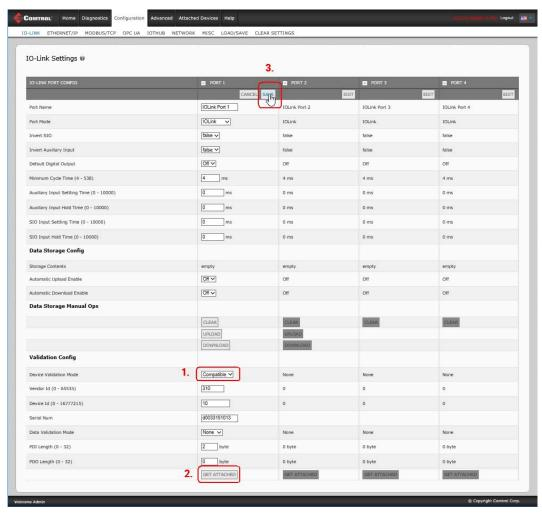
5. Click the SAVE button. If the wrong or incompatible device is connected to the port, the IO-Link port LED flashes red and no IO-Link activity occurs on the port until the issue is resolved.
