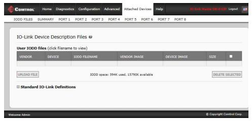
The IOLM provides 15790K of space to store IODD files. The IOLM includes the following default IODD files, which cannot be deleted.
