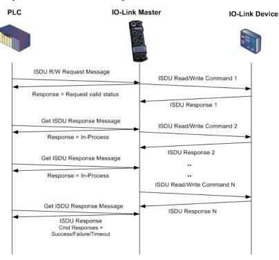
Multiple Command ISDU Non-Blocking Process
